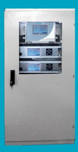
Agasthya 2013 series BI7220 Producer Gas Analyzer is designed considering the flexibility required in the environments that characterize syn gas and bio-mass applications.
